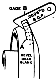
FIG. 12.—MARKING DEPTH ON BEVEL-GEAR BLANK.
